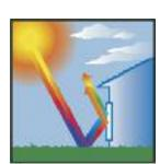
Low-E glass filters longwave radiation from the sun. This reduces heat gain in the summer, keeping your home cooler.
